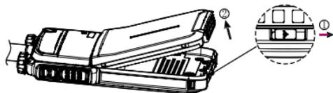
Step 2 Loosen the screws fixing the SIM card cover, open the cover, and then place the card into the slot properly, as shown in the figure below.
